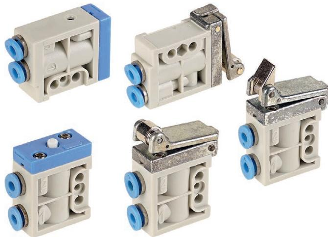
Series of poppet microvalves mechanically operated. Connections with integral 4 mm push-in fittings. According to the application you can choose between the version with bottom connections or side ones.
