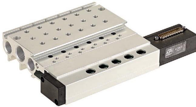
Sub-bases with fix position for A2 series valves, with standard 25 poles SUB-D connector, can be mounted on DIN EN 50 035 guides.
