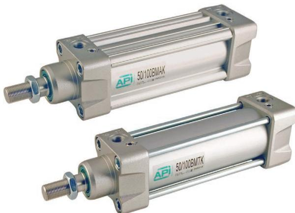
Series of cylinders conforming to ISO 15552 standards, that can be supplied with two different shapes of the barrel: BMA type with "T" and "C" grooves allowing to use the flush-mounted magnetic switch, and the BMT type with round tube and tie-rods.
