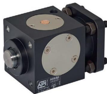
Series of dynamic locking-rod units for cylinders ISO15552. The piston-rod brakes series ABK can be supplied normally closed. The peculiarity of this series is to lock the cylinder piston-rod while moving and to hold it still even in presence of pressure in the chamber.
