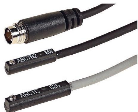
The magnetic reed switches are magnetic sensors responding to the presence of a magnetic field. When mounted on a cylinder tube they detect the presence of the magnetic field generated by the magnet set on the piston and so of the piston itself. This information is used to signal electrical circuits as required.
